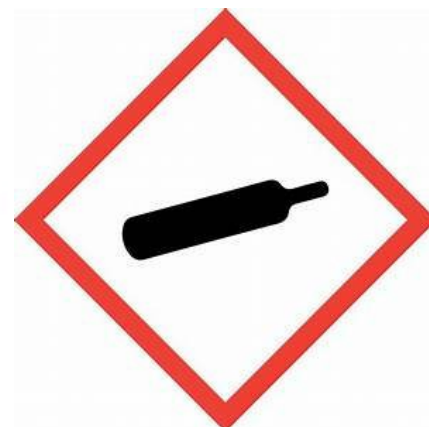
Gas Under Pressure
